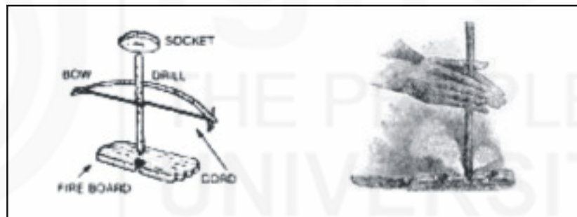
Fig. 4.17: Bow Drill and hand Drill
